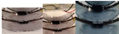
Figure 2: Images of plastic material after exposure for 4 days with 0.5 – 0.6 mW/cm 2 of UV light
